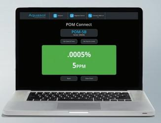
**GREEN** indicates that the current measurement is lower than the "Lower Alarm Limit."
