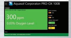
When the oxygen content reaches the operator set TARGET PPM level, the numerical value will display on a **GREEN** screen, a visual signal that welding can commence per the operator's instructions.
